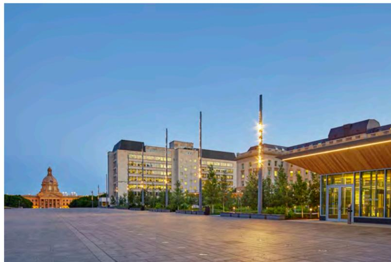
**Figure 117:** Edmonton Legislature Grounds: The plaza is illuminated to high levels (20 lux) for festivals, but with many small fixtures, allowing each head to appear as sparkle instead of the glare that would come with fewer, larger fixtures.
