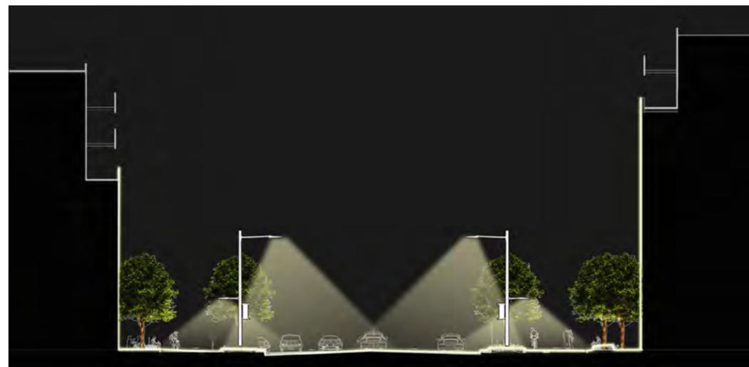
**Figure 123:** Pedestrian and street lights section
